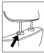
The height of the front seat head restraints can be adjusted. Pull the restraint up to raise it. To lower it, press the button, located on the top of the seatback, and push the head restraint down.
